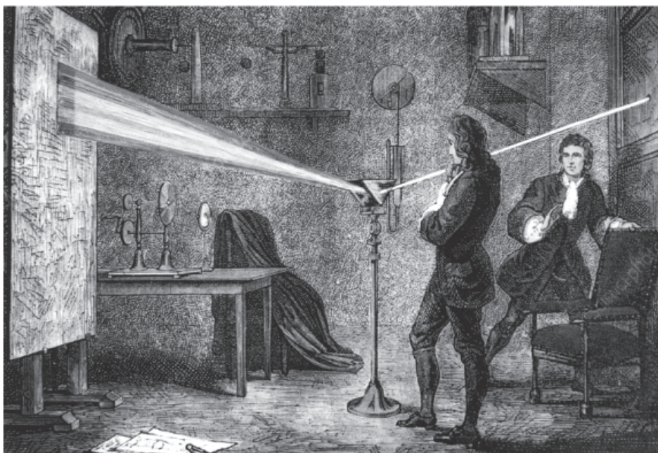
Fig 3: Sir Isaac Newton’s experiment with prism and dispersion of light(Image Courtesy: Google)
